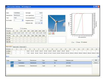
The equivalent noise level is calculated using the wind speed statistics at hub height. Wind speeds at 10 meter height are automatically converted into wind speeds at hub height using the terrain roughness.
