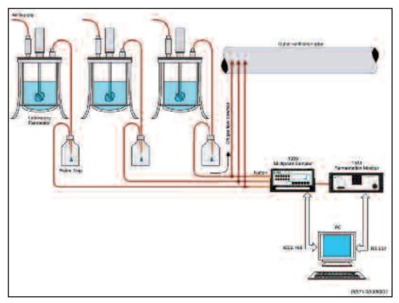
Fig. 3 The diagram shows samples being drawn from three fermentation vessels. Up to 12 similar analyses can be performed simultaneously using one 1309 and the PC Software supplied with the 1313
