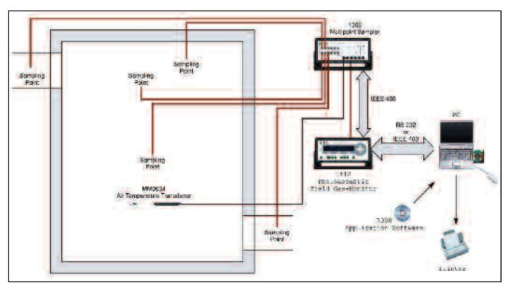
Fig.2 A typical sampling system, shown with an application example. The diagram shows 5 sampling points, for clarity. Up to 12 similar analyses can be performed simultaneously using one 1309. Application Software 7300 gives control of all the functions of the system.
