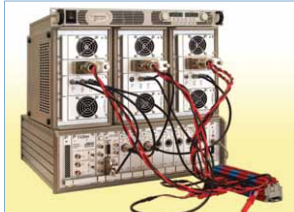
A T3Ster system with three high current boosters and an external Agilent power supply aimed at high current applications such as IGBT measurements.
