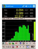
FFT based Octave Analysis and 3 mode of Vibration Measurement
