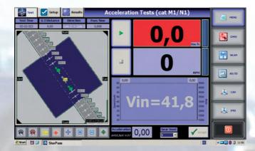
uses both the code and phase signals to determine the vehicle position (carrier Phase Doppler technique), while the speed calculation is refined via a Von Kalmann filter optimized for dynamic performance.
