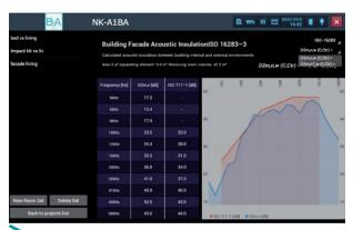
The program finally reports a test proof for building acoustic in conformity with standard UNI-EN ISO 16283, and UNI-EN ISO 140. It shows a graph with the curve trend as from the standard (light red) and the curve trend from measurements.
