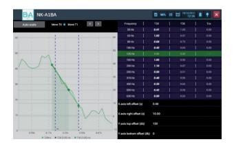
The program shows for each frequency (from 50 Hz to 5 kHz) three calculated values: T20, T30 and Txx. User can set Txx edges: T0 and T1. The vertical blue dashed lines identify T0 and T1 along the curve; in the meantime, the calculated Txx for the specific interval appears in the table.
