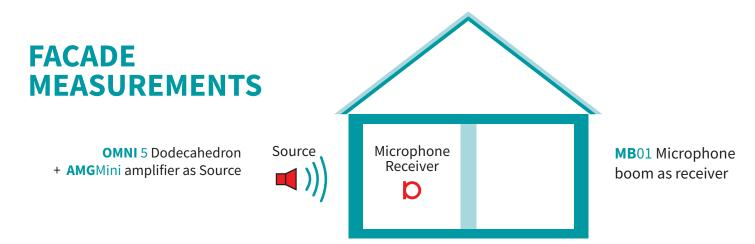
Façade measurements can be performed by means of a source external noise and a microphone receiver as required by the standards: UNI EN ISO 140-5 Field measurements of airborne sound insulation of facade elements and facades, UNI EN ISO 16283-3 Façade sound insulation and UNI EN ISO 3382-2 Reverberation time in ordinary rooms.
