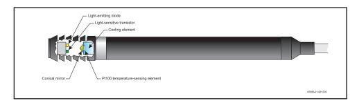
surface. The Pt100 sensor registers this dew- point temperature.
