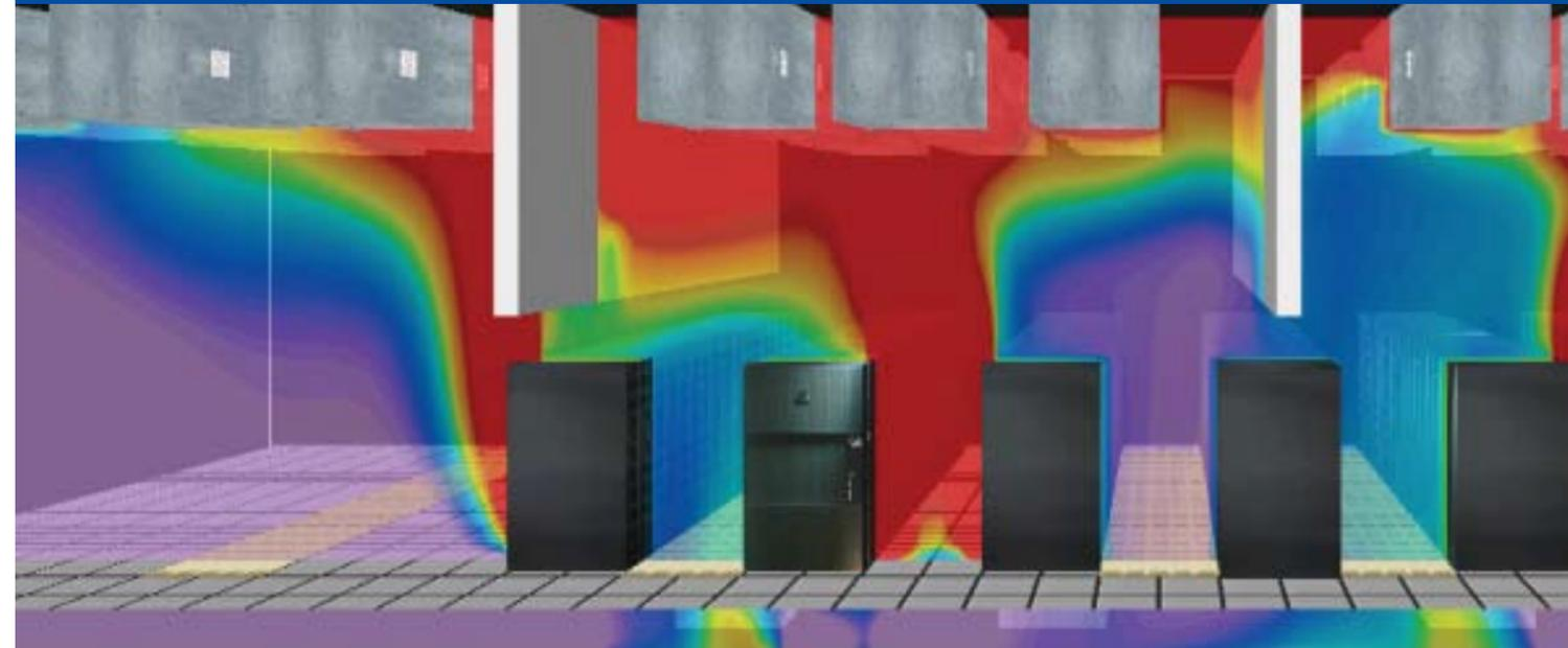
We provide a computational test bed to evaluate airflow and thermal behaviour of current and future data center designs, and operational changes. Armed with this vital information, you can quickly and easily:
