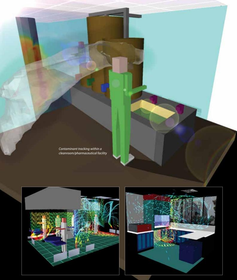
"We have found that applying airflow modeling technology in the design of our clients' cleanrooms has proved beneficial for reduction of capital costs, verification of design and optimization of operations, and has led to new design innovations, such as new concepts for 300mm manufacturing environments."
