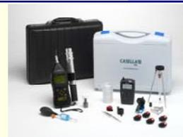
Shows P104124 kit comprising Microdust Kit, Apex Starter kit, Apex Lite pump and pre weighed filters
