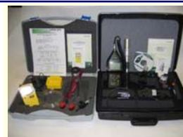
Shows P104105 kit comprising Microdust Kit, Apex Starter kit, Apex pump and charger
