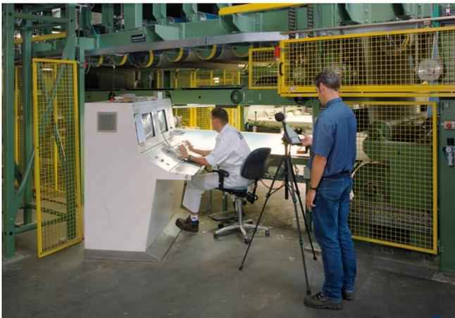
Figure 1: Noise measurement at the workplace
