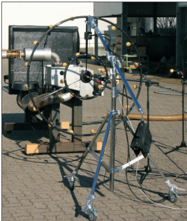
Localization of sound sources on a screw-type compressor using a double-circular array
