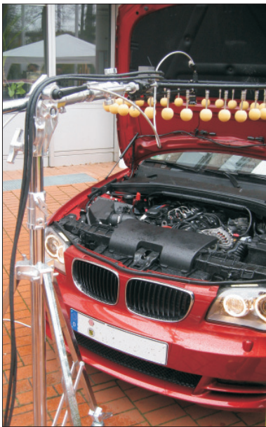
Localization of sound sources in the engine compartment of a passenger car
